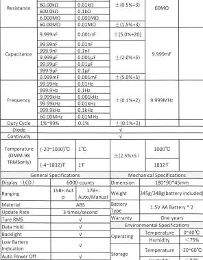
Humidity <80% Safety Specifications EN 61010-1: 2010; EN 61326-1: 2013; FCC Part 15 Subpart B: 2016 Standard Accessories Battery \* 2pcs; Test Lead \* 1 pair
